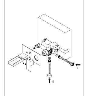
Please check that your pressure is suitable for this product before installation, details can be found on our website, recommed minimum working pressure: 0.5 bar, maximum working pressure: 3 bar
